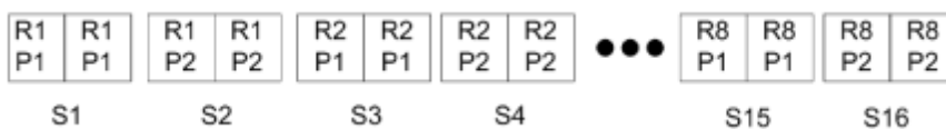
Figure 1: Example of single-record imposition using Repeat Gangup for 8 records, 2 pages per record, 1 row x 2 columns layout, simplex. R = Record, P = Page, S = Sheet.
