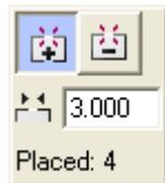
Nicks are small pieces of substrate that are not cut by the table and thus create interruptions in the cut path. As a result, the cut design will stay attached to the substrate. Nicks may be present in the design, but the nick tool allows you to add or remove extra nicks that guarantee tiles to stay connected. You can specify the size of the nick in the box. Click the cut path and add or remove nicks as you wish. When exporting, the position and size of the nicks will be saved in the .cut file.
