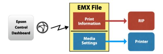
After the media are registered in the printer, the system is ready to use with the Fiery XF RIP software.
