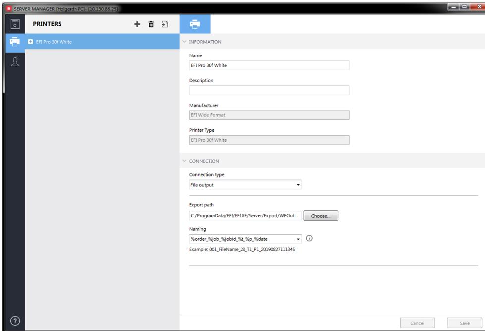
When set up this way, the Fiery XF server RIPs the job and creates a \*.bco file. Use the EFI Print Control Utility to select the \*.bco file and print the job. For more information on how to use the EFI Print Control Utility, see the printer's Operator's Guide.
