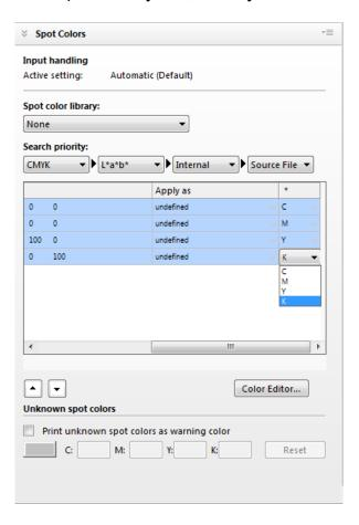
The spot color table shows which screen angle is used for each color. The default setting for all spot colors is black, but you can select the screen angle of any other process color in the "\*" column. Scroll to the right to view this column.
