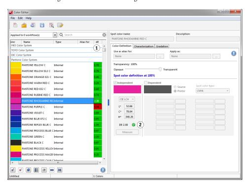
The delta E value indicates how accurately the spot color can be reproduced.
