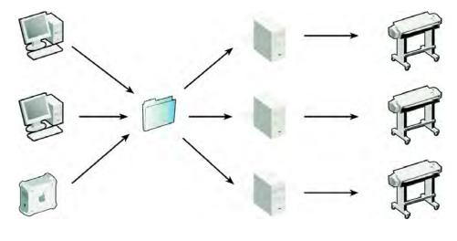
Example of load balancing using different workflows
