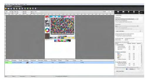
If color accuracy is approved, the job receives the status "Verified". In this case, the verification procedure is complete. If color accuracy could not be approved, the job receives the status "Verification failed".
