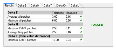
A green check mark indicates that the overall measurement is within the tolerance limit. A red cross warns you if a measurement exceeded the maximum tolerance values.
