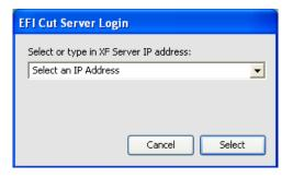
To log on to a specific EFI XF license server, choose an IP address from the drop-down list box, enter an IP address manually or type "localhost" if the EFI XF Server and Cut Server are on the same computer.
